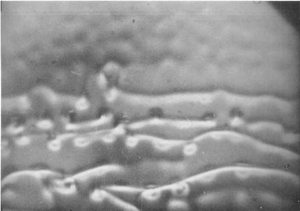
FIGURE 10. Sulphur dioxide-water system viewing perpendicular to interface. Surface of lower half of photograph covered by oleic acid monolayer, upper half by natural contaminant. \Delta P = 0.16 atm, field of view approximately 14 \times 20 mm.
